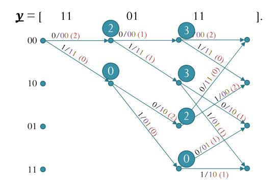
Each circled number at a node is the running (cumulative) path metric, obtained by summing branch metrics (distance) up to that node. Here, it is simply the cumulative distance.
